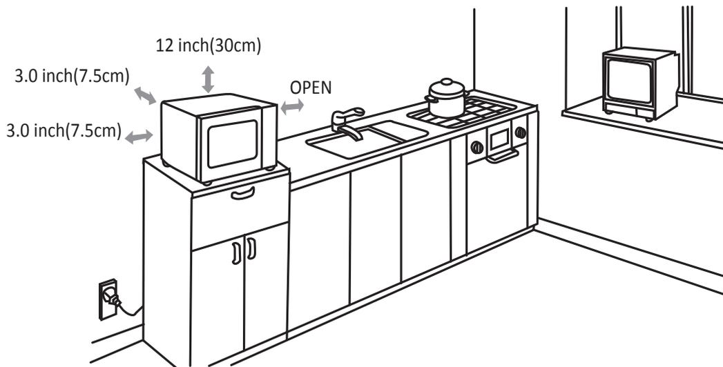
1. Select a level surface that provide enough open space for the intake and/or outlet vents. A minimum clearance of 3.0 inches (7.5cm) is required between the oven and any adjacent walls. One side must be open.
