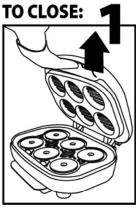
Lift handle vertically to clear lock tab.
