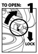
Gently open until hinge drops into locked position.
